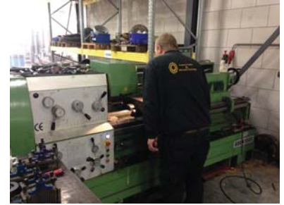
Manufacturing of a Pump-shaft
